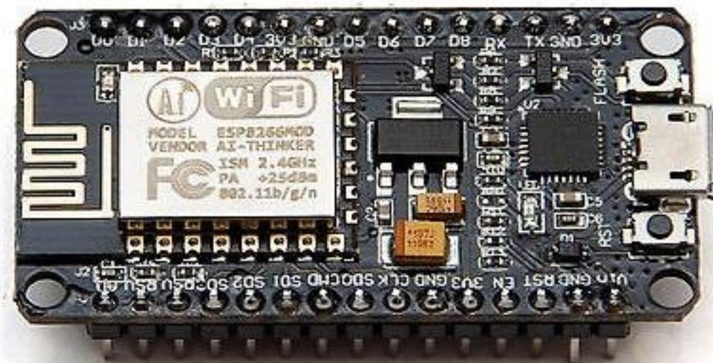
**Fig 1.5:** NodeMCU 12E ESP8266 Module
