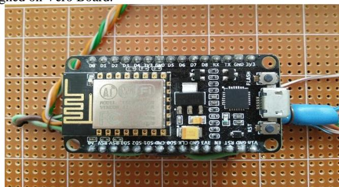
Fig 2.3: Circuit on Vero Board.
