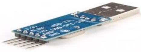
**Fig 2.7:** USB to TTL Converter
